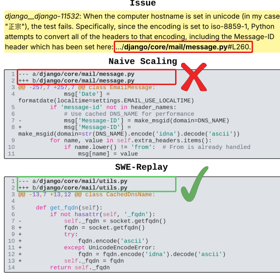
Figure 7. Example of fixing failure due to inadequate exploration. Naive scaling fixated on message.py (incorrect), whereas SWE-Replay successfully branched out to explore utils.py (correct).
